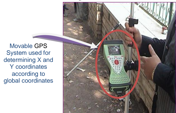
Plate (2): Movable GPS used for measuring the coordinates along sides.
